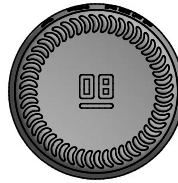
VIEW ON BASE SHOWING EMBOSSED MARKINGS & STANDING AREA EMBOSSED WITH STIPPLES.
